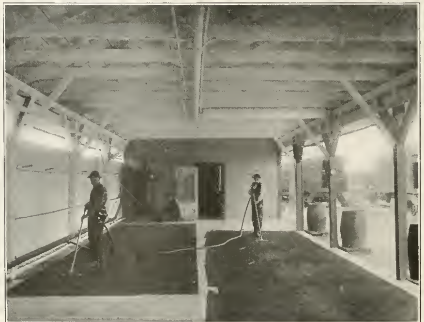
Carpets, rugs, aisle strips, mats, cushions, hassocks, and mattresses are cleaned either with compressed air or by vacuum system.
